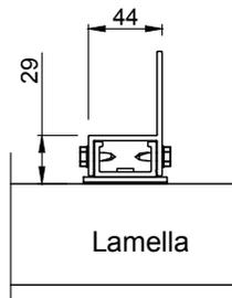
Lamella, mounting profile, frame and bracket
